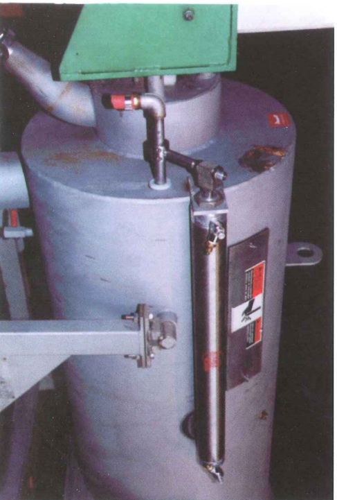
ABOVE AND BELOW: AN AIR CYLINDER ACTUATES THE TRAVELING SPRAY RING MECHANISM
